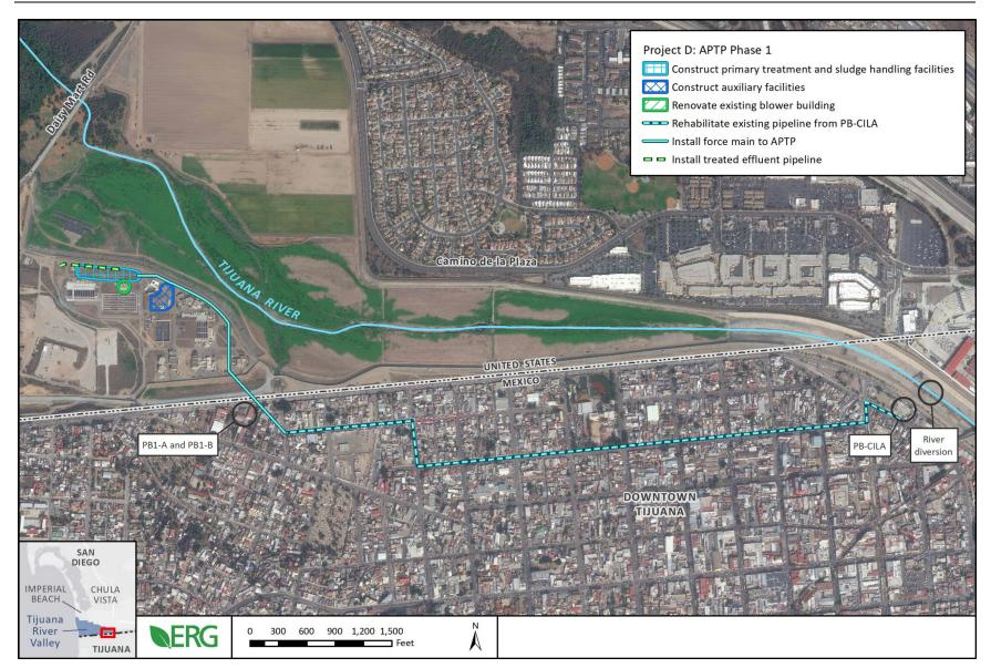
Figure 2-11. Project D (APTP Phase 1) – Locations of Project Components (2 of 2)
